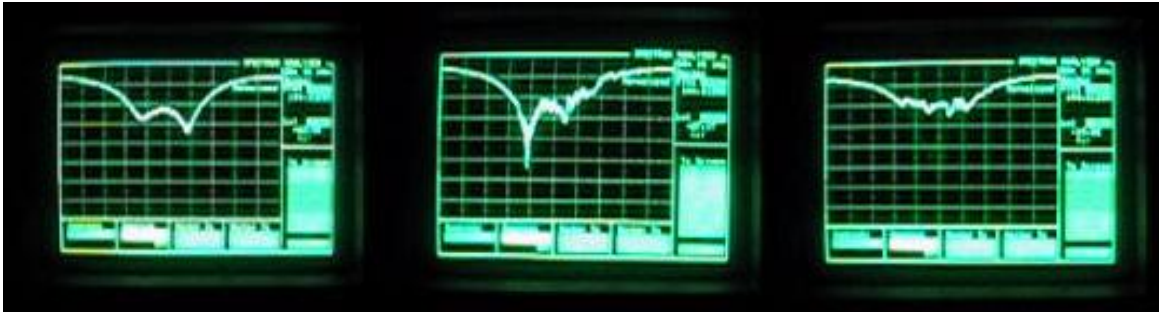
Figure 3 - Three screen shots show the way the return loss plot jumped around
