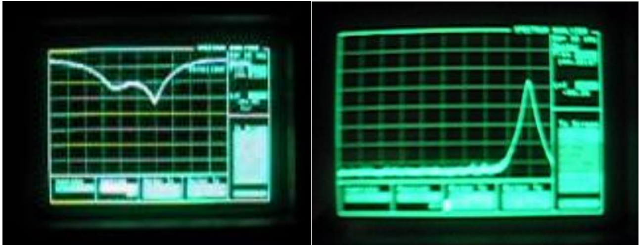
Figure 5 - After the fix we had a nice stable return loss plot, shown on the left side figure. The right side figure shows a spectrum plot of the signal coming into the receiver with the transmitter keyed. The plot is centered on the receive frequency and the attenuated transmit carrier is shown on the left. It is at around -46 dBm. There were no transmitter induced parasitics on the receiver frequency.
