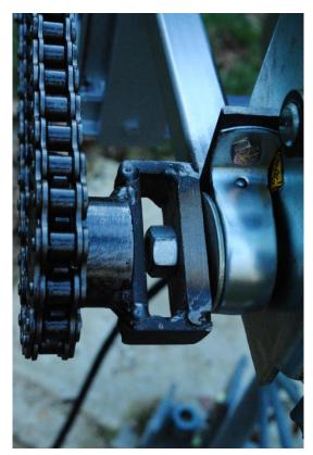
The sprockets used in this project are available at Tractor Supply or similar hardware store. They are designed to be used in a keyed configuration or suitable for welding as illustrated to the left. Unfortunately the winch shaft is not "keyed" in a manner accommodating these sprockets.
