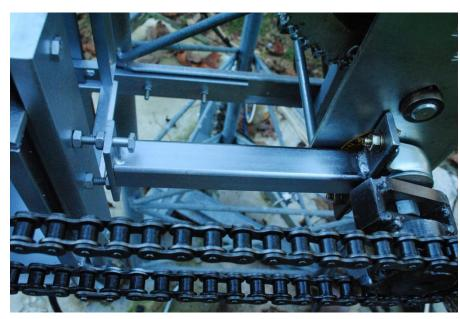
To the left is a close-up of this important restraining member. The left side is somewhat floating, with force in +/- x directions being provided by the positions of the nuts on the two grade 8 bolts. If detached on the left, the assembly will just free-rotate on the winch shaft bearing to a vertical position. All the force is in the +/- x directions, provided everything is lined up <sup>⊚</sup>.
