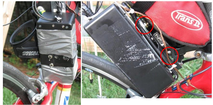
Duct tape field repair after a critical attachment holding the APRS tracker to the bike failed 10 miles earlier when a lock washer didn't (do it's job)!
